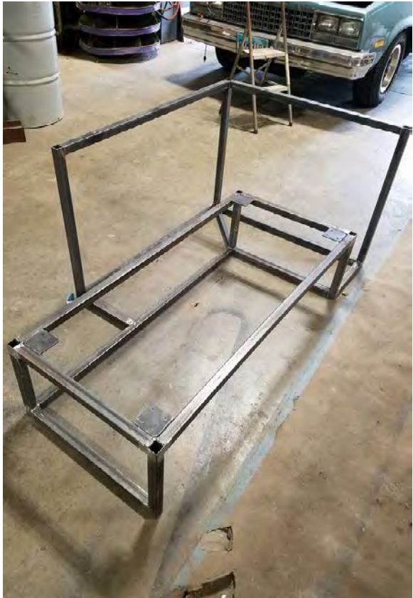
The seat was built and upholstered by Orange Chair in Cincinnati. The frame was welded by A.J. Pate and powder coated by Leonard LeFevre.
